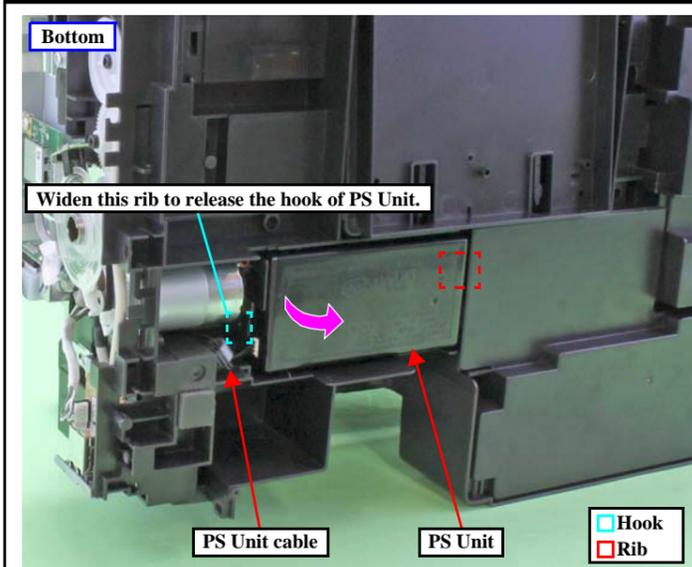
**!** Be careful not to damage the rib of the Frame Base when widen the rib to release the hook of the PS Unit.
