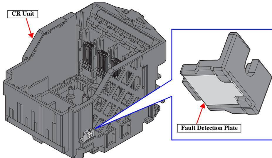
Figure 1-4. Fault Detection Plate
