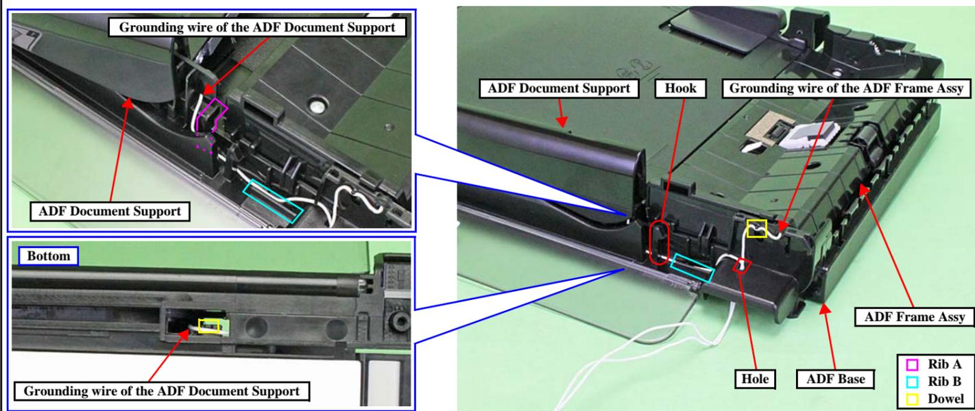
Rotate the grounding wire of the ADF Frame Assy and ADF Document Support(x2) as follows.
