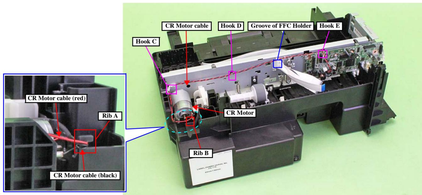
Route the CR Motor cable as follows before installing the Shield Plate.
