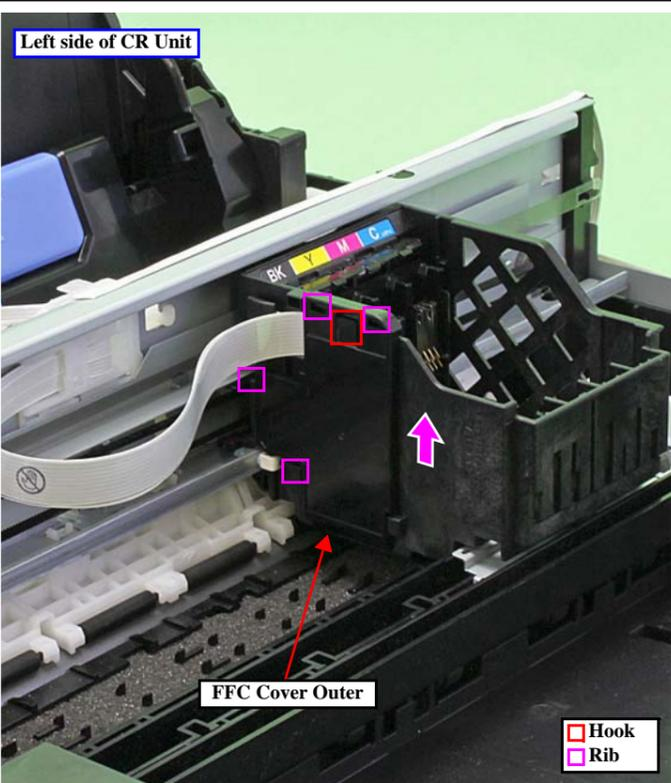
Slide and remove the FFC Cover Outer in the direction of the arrow while releasing the hook.
