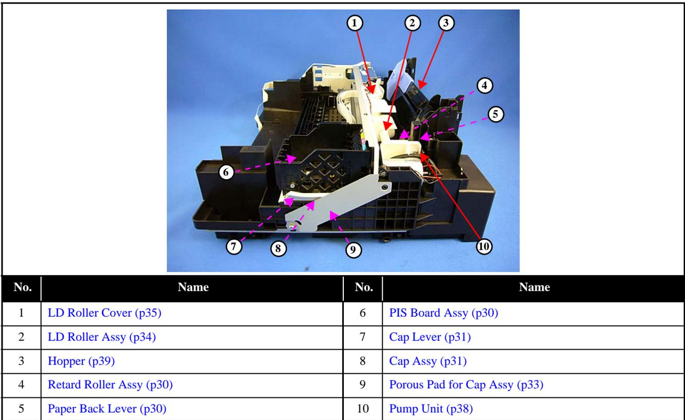
Figure 2-4. Printer Mechanism: Right
