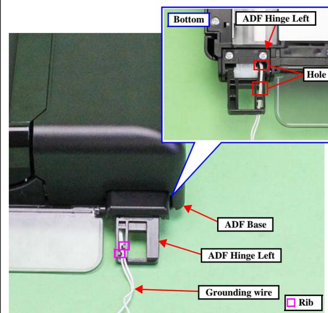
Route the grounding wire (x2) of the ADF Frame Assy/ADF Document Support through the ADF Hinge Left as follows.
