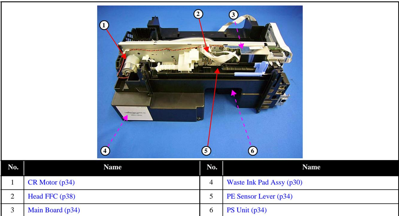
Figure 2-6. Printer Mechanism: Rear
