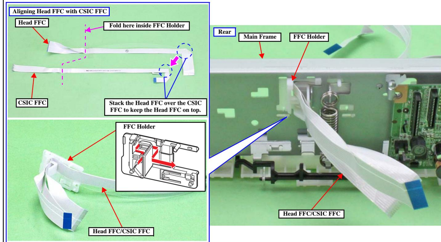
Align the Head FFC and CSIC FFC, and then route them through the FFC Holder as shown in the figure above.
