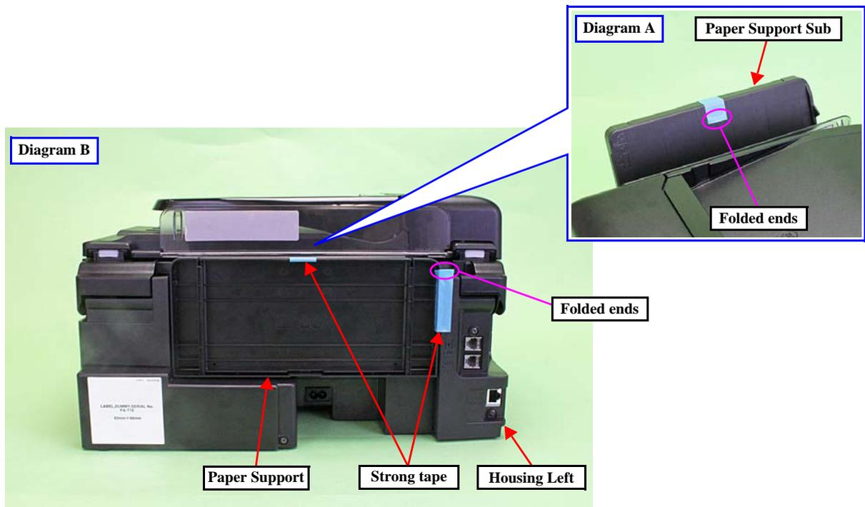
Figure 6-3. Securing the Paper Support/Paper Support Sub (Multifunction Printer)
