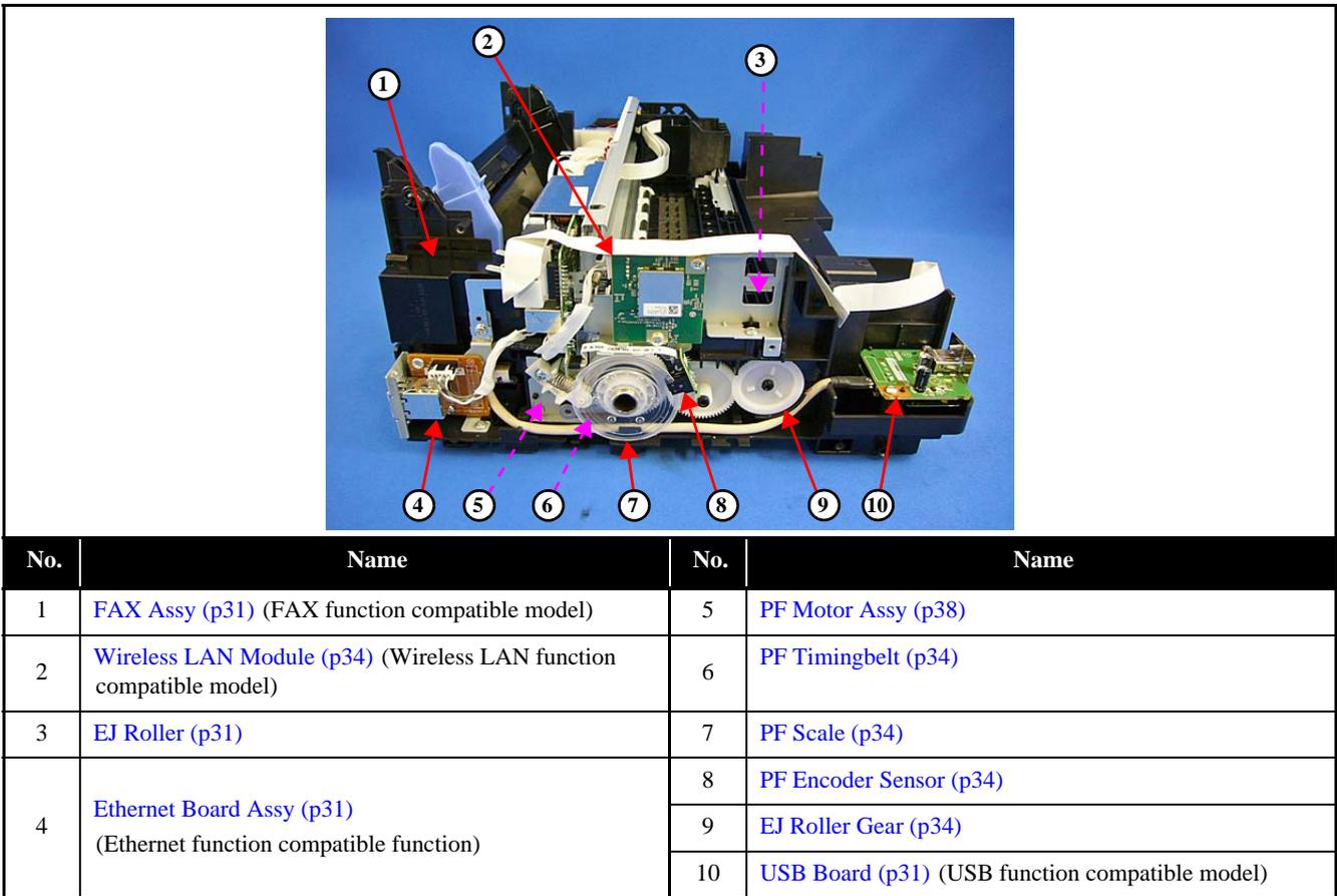
Figure 2-5. Printer Mechanism: Left
