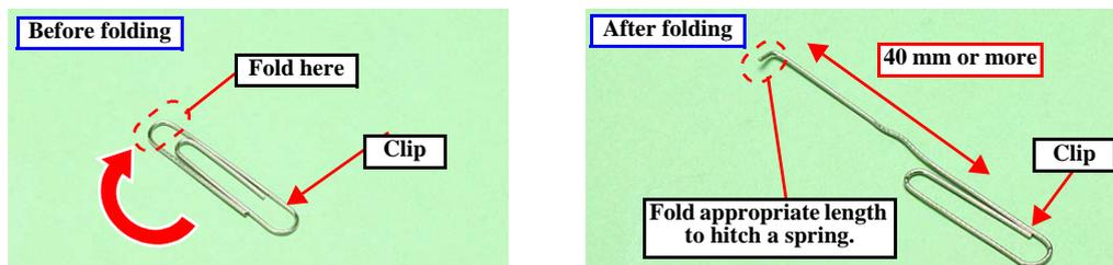
Figure 2-1. Making the Spring Hook Jig
