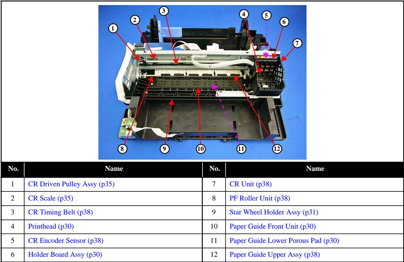
Figure 2-3. Printer Mechanism: Front
